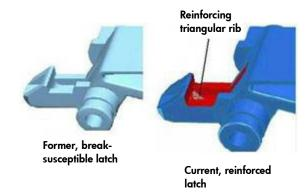
Fuser latch countermeasure diagram
